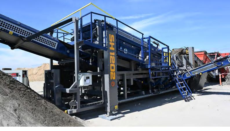
Because of the handy format and wide application possibilities the SH 1202 will undoubtedly increase the versatility of your fleet of machines. Use it as a standalone screen, together with the crusher, a screening plant or in a stationary production line to split a fraction, instead of stopping the entire application for change of screening meshes.
